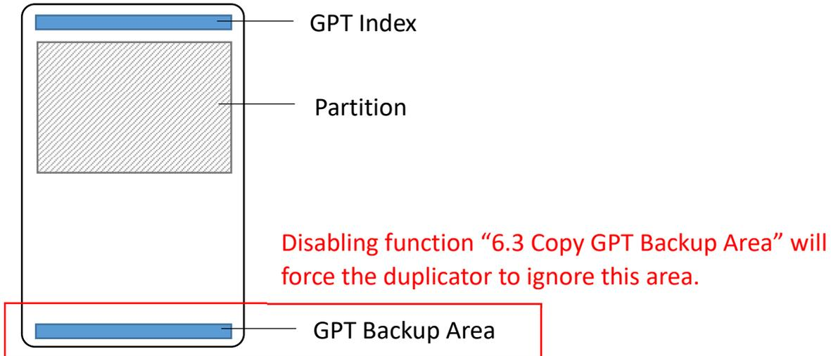
**Caution** If function is disabled, the target HDD will reconstruct the GPT Backup Area by Windows system. It may require the HDD to restart in order to work.
