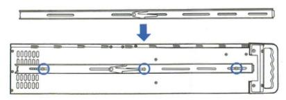
Now put the center slide right next to the rackmount chassis. You should be able to find screw holdes on both sides of the chassis. Holes are used for mounting the center slide. Later, the center slide will be use for attaching the sliding rail.
